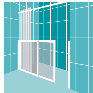
Option 2 One set of sliding doors hung off one side latching on opposite wall
