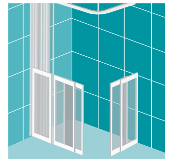
Option 6 Fixed 400mm half height panel, floor to ceiling pole with pair of sliders meeting a return pair of sliders on the corner
